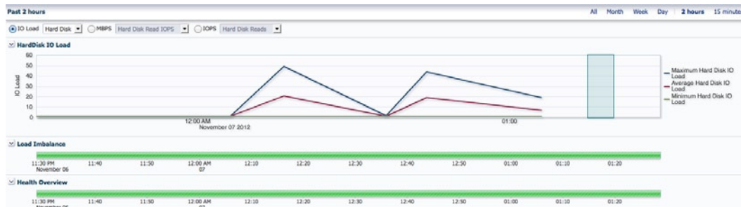
Figure 14-5. Hard disk I/O load on storage cells
